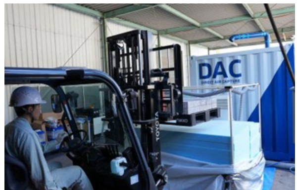
Placement of pavement blocks in the Carbonation Curing Chamber
